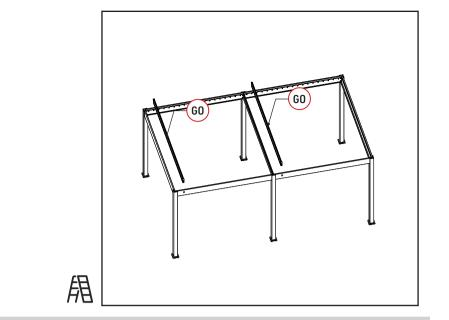
Fasten rubber plugs on both ends of the louvers
