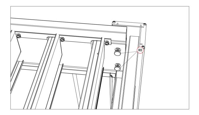
After confirming the dimensions, then fix the expansion bolts on the plate.
