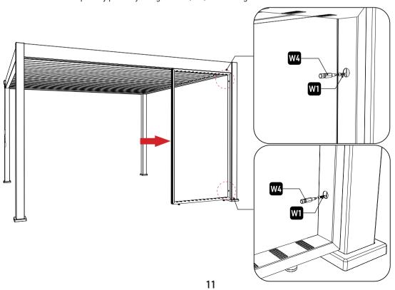
Fix the upper frame of the privacy panel by using screws(W1) as the diagram shows below.
