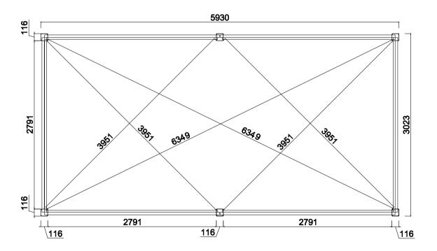
3D FOOTING MEASUREMENT (dimensions in mm)
