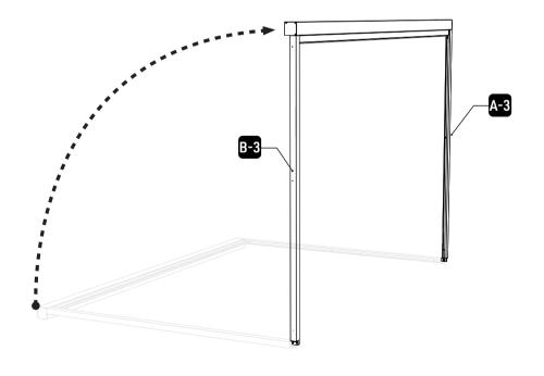
Put the frame up and make sure the outer face of wind screen box align with outer face of beam.
