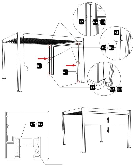
Please make sure the foam strip on the sides of A-2/B-2 can be inserted into the U groove of the wind screen's frame.
