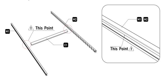
After inserting the E1, please use the screw(W1) to fix the two ends of E1 onto the frame.
