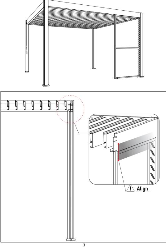
Adjust the adjustable bases again to make sure they just stand on the ground.
